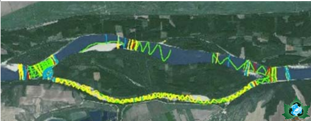
Fig.5. Single beam measurements locations on the Old Danube and Epurasu branches
