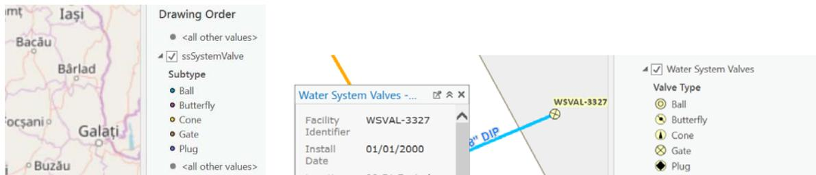
Fig. 6 –Subtypes Defined for Water Network in ArcGIS Pro (according with [15], [16])
