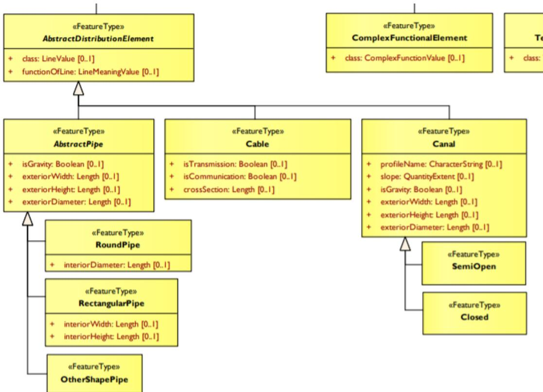
Fig. 9 - Extract from UtilityNetwork ADE – UML Model (according with [21])
