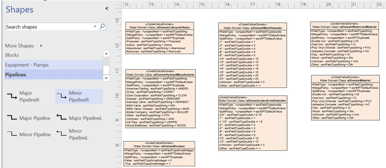
Fig.5 – Defining Domains for Water Network in MS Visio (according with [15])
