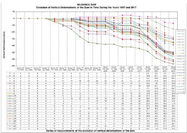
Fig. 5. Evolution of Vertical Deformations of the Dam During the Years 1997 and 2017
