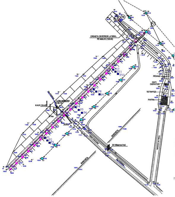
Fig. 4. Dam body plan view with the location of the measuring installations.
