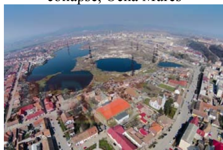
Fig. 8 Lakes formed above Ocna Mures exploitation sites
