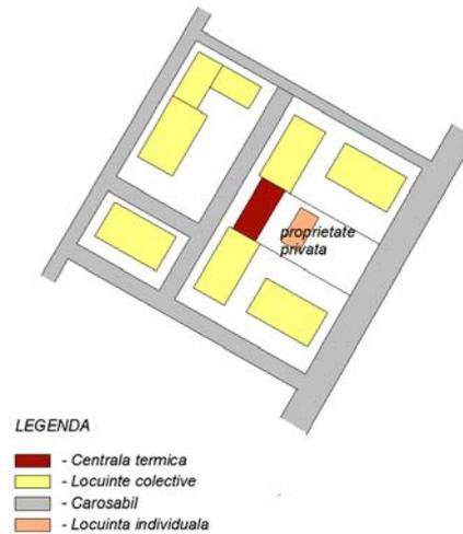
Fig.11: Example of central heating plant location in the quadrant of collective dwellings
