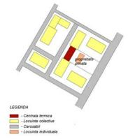
Fig.5: Example of central heating plant location in the quadrant of collective dwellings
