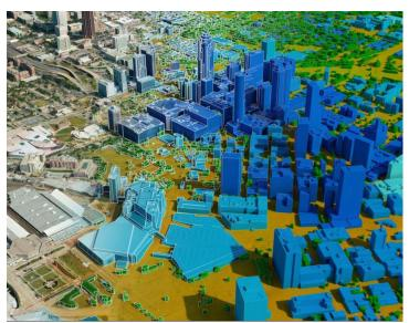
Fig. 4. 3D polygons - Level of detail (LOD 1.3) (image courtesy of DigitalGlobe)
