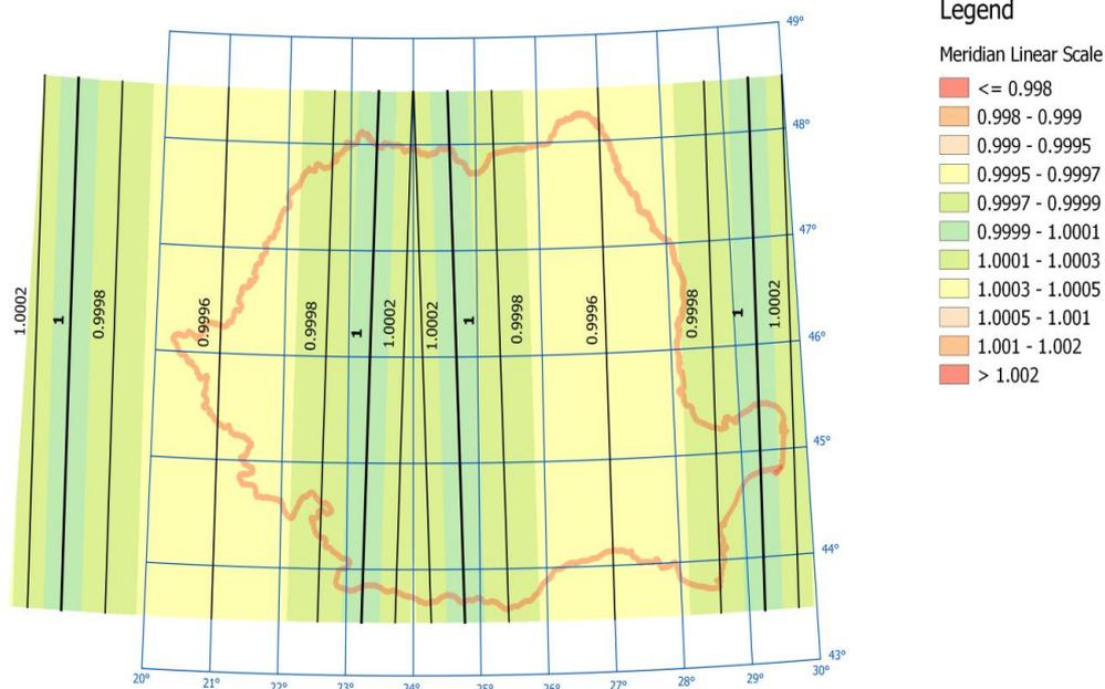
Fig.10. Linear deformation map of the meridians in the projection UTM
