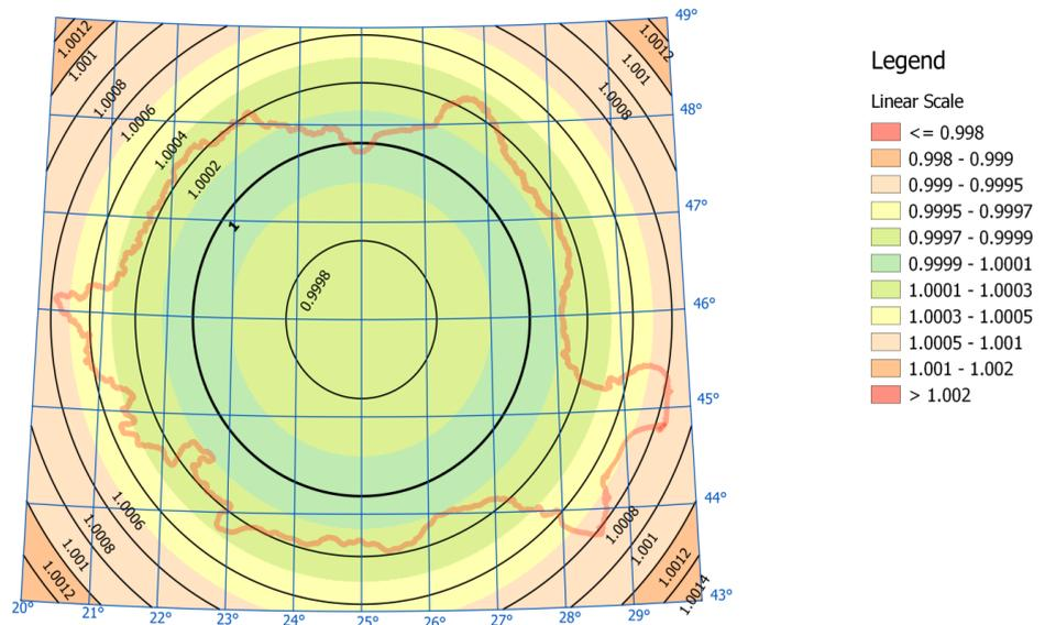
Fig. 4. Linear deformation map of the meridians in Stereographic Projection 1970
