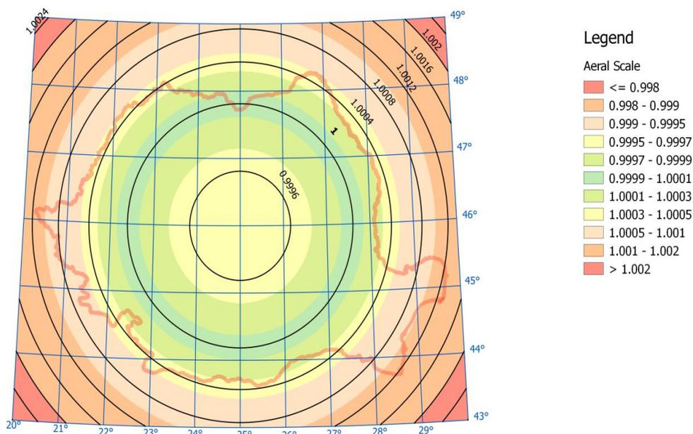
Fig. 8. Map areolar deformation module in Stereographic Projection 1970
