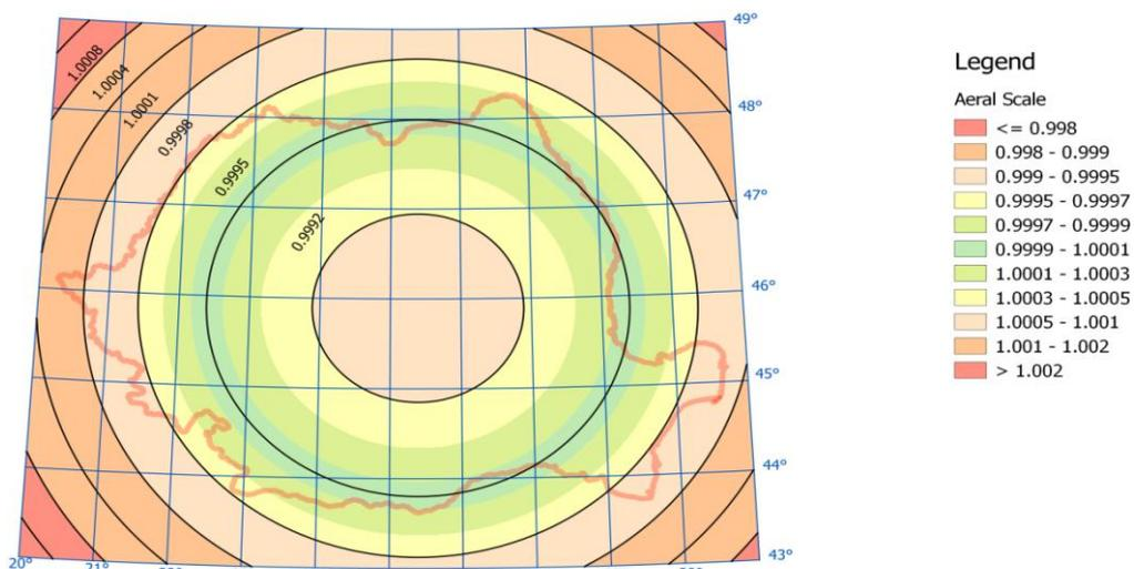
Fig. 7. Map areolar deformation module in Stereographic Projection 1930(1933)
