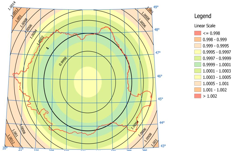
Fig. 3. Linear deformation map of the meridians in Stereographic Projection 1930(1933)
