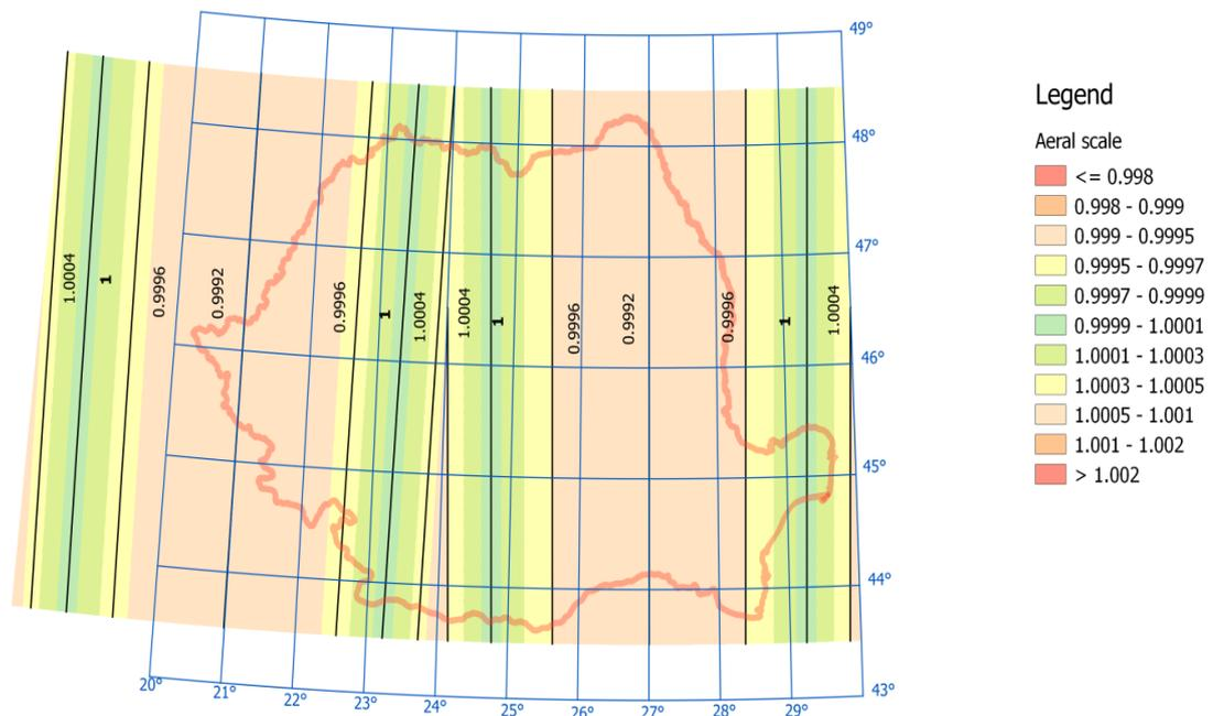
Fig.11. Map of the areolar deformation module in the projection UTM
