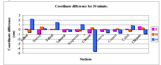
Figure. 9. The difference of the calculated coordinates and initial coordinates for 30 minutes
