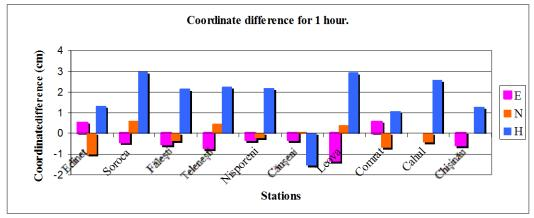
Figure. 8. The difference of the calculated coordinates and initial coordinates for 1 hour
