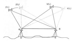
Figure. 4. Relative position with triple difference [1]
