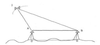
Figure. 2. The relative position with simple difference [1]
