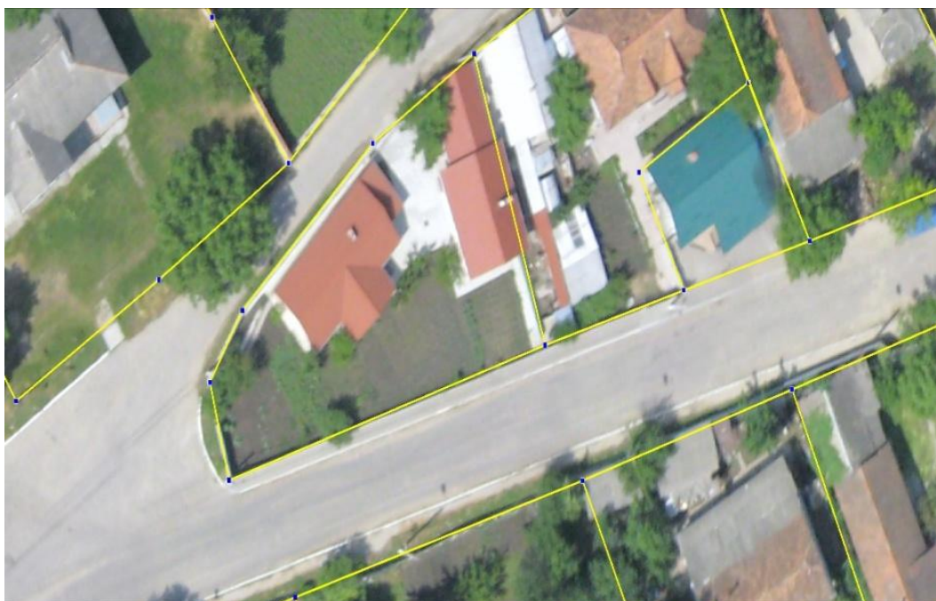
Figure 6. A fragment of the cartographic material of Panasesti village, obtained with the help of the PAMS system, which serves as a basis for vectoring the real estate parcels.
