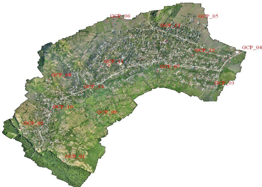
Figure 3. Orthomosaic of Panasesti village with GCP points representation for georeferencing in the Moldref 99 system Source [1]
