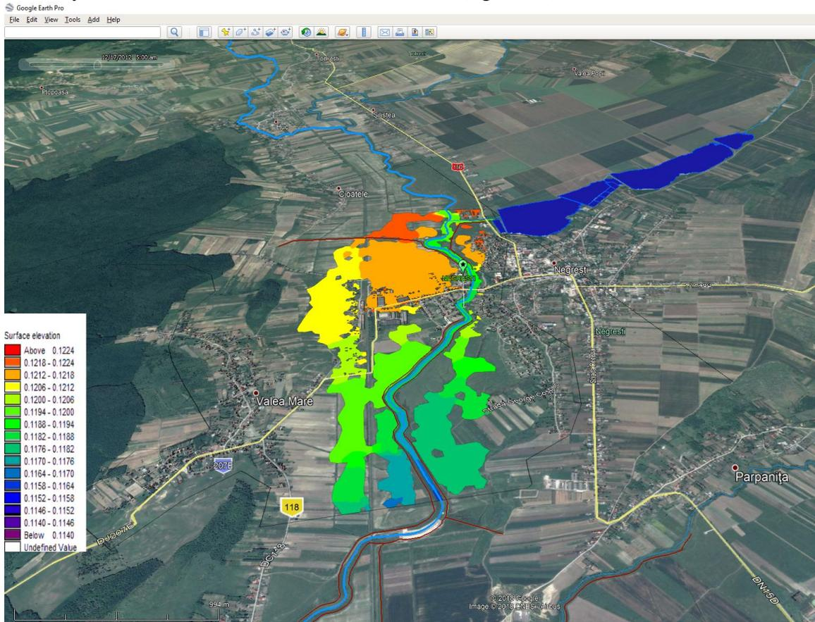
Fig. 10 - Runoff simulation extents on Google Earth
