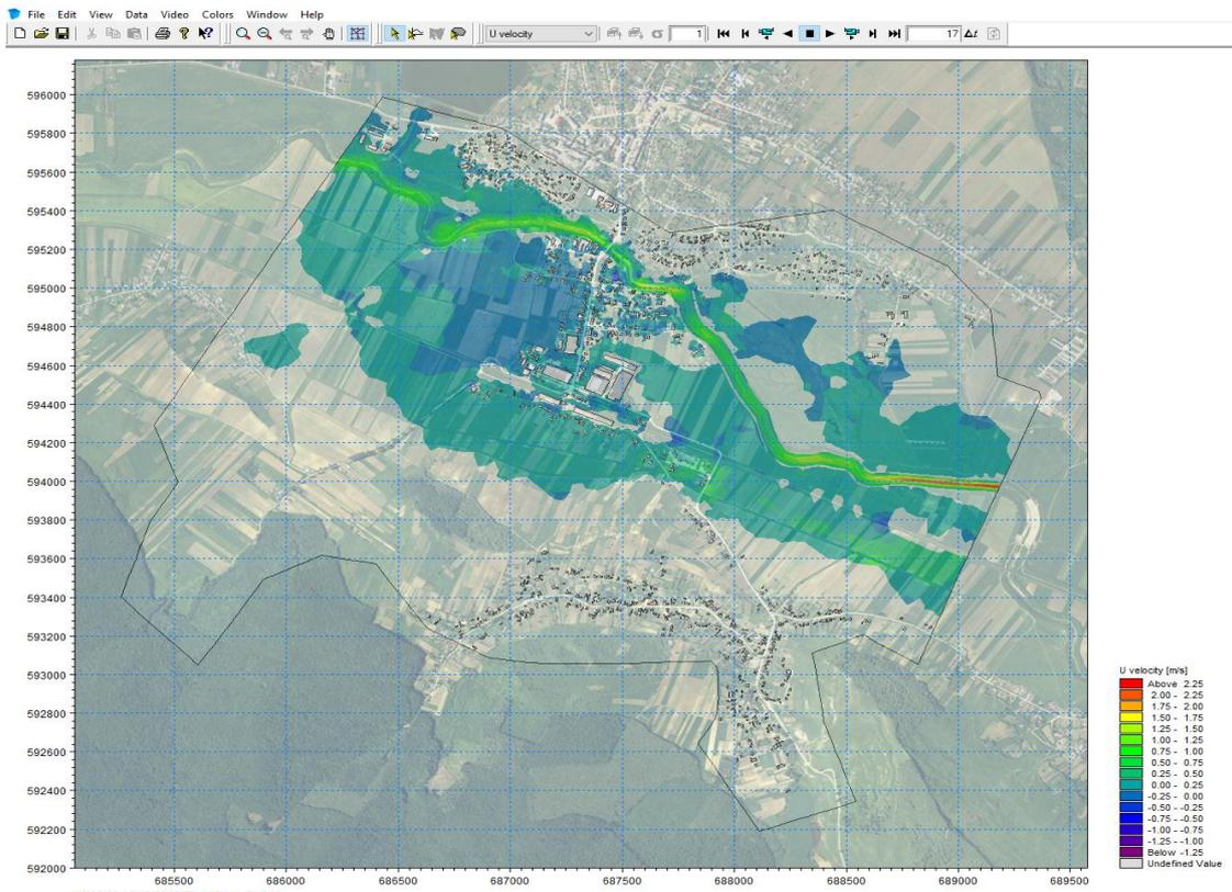
Fig. 9 – Maximum velocity of water – horizontal dimension
