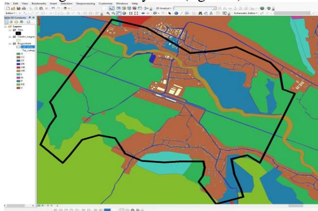
Fig. 1 – GIS data of streets, buildings and roughness coefficients
