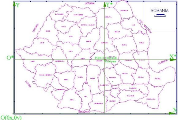
Fig. 8 The position of the central point in the stereographic projection on the single secant section Braşov
