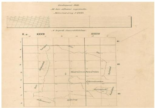
Fig. 3 Extract from the map sheet edited at a 1: 2880 scale from 1913 and realized with the stereographic projection system with the tangent plan in Budapest
