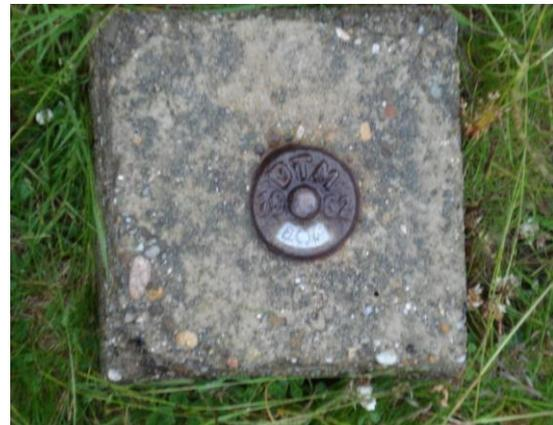
Fig. 5 Geodetic Beacon and Stone of Sălâne
