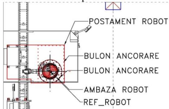
Fig. 6 Robot specific elements
