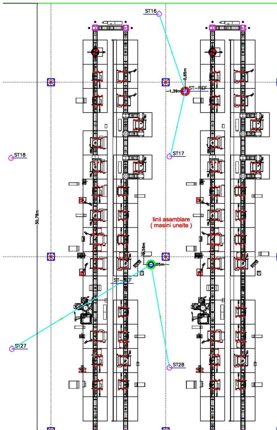
Fig. 3 Equal distribution of stationary points in the design of industrial facilities of long lengths
