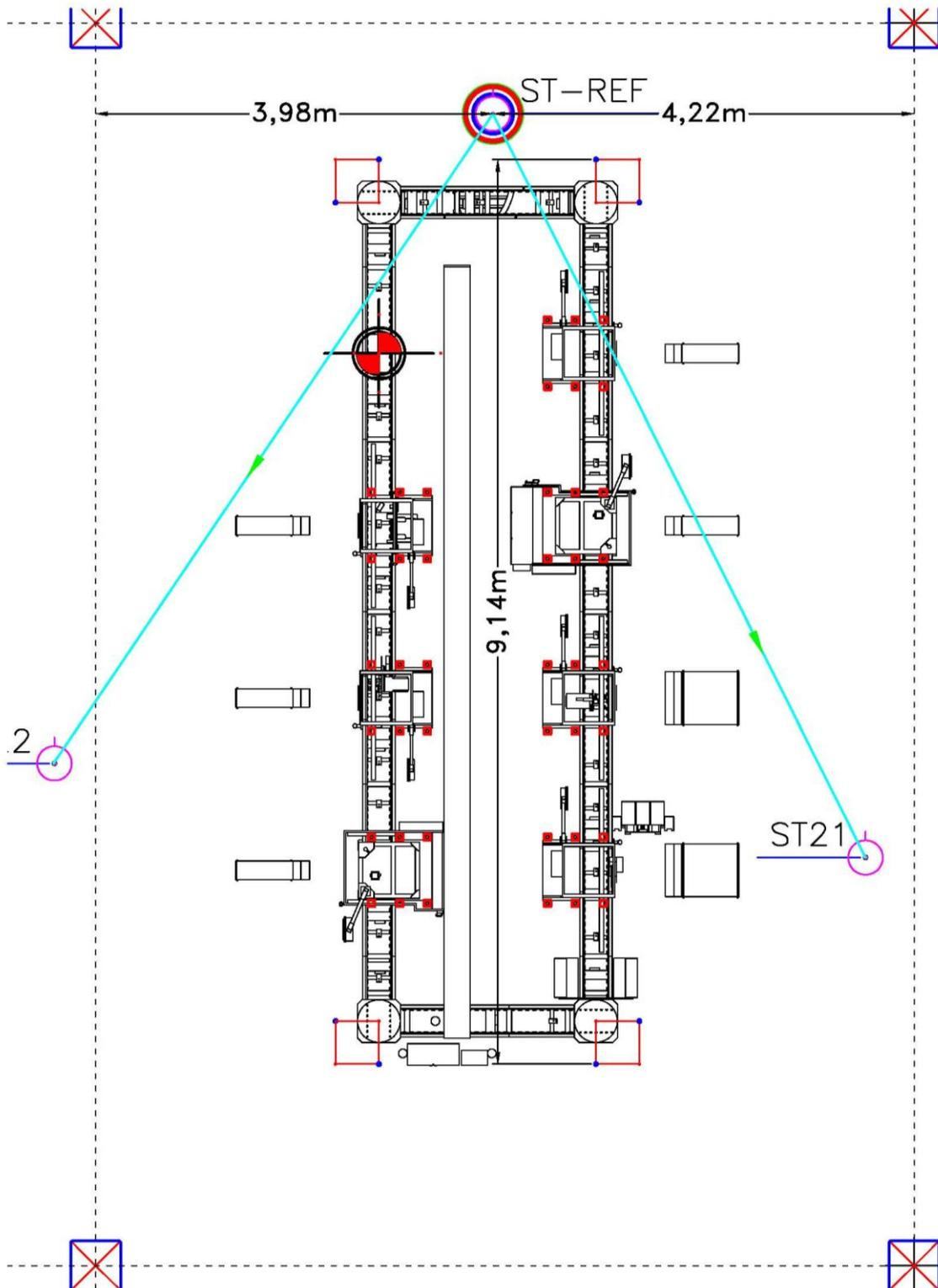
Fig. 2 The procedure for determining the location of the topographical instrument
