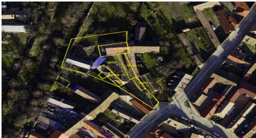
Figure 9 – Site and position plan incorrectly placed
