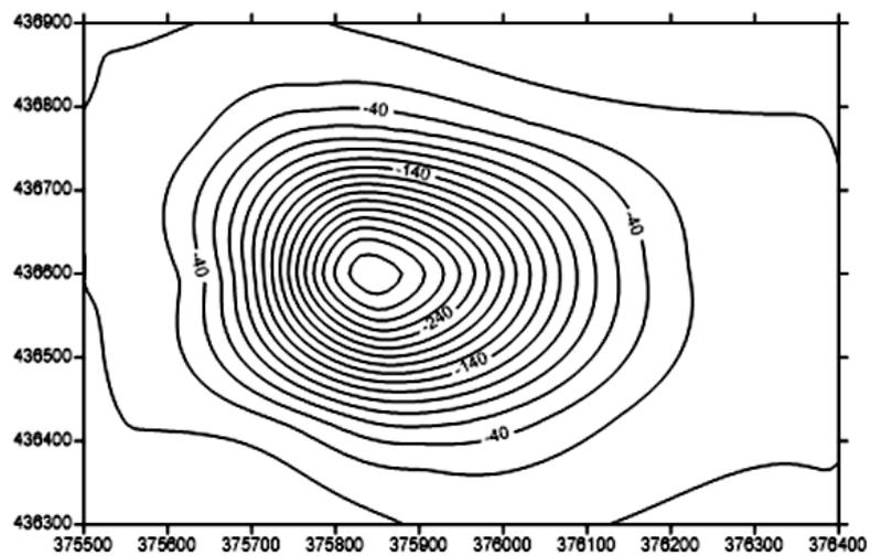
Fig.6. Representation through equal subsidence curves of the diving bed
