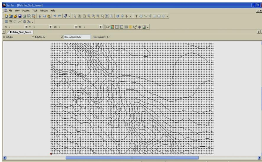
Fig. 4. The model of a .grid file required to create the digital terrain model.
