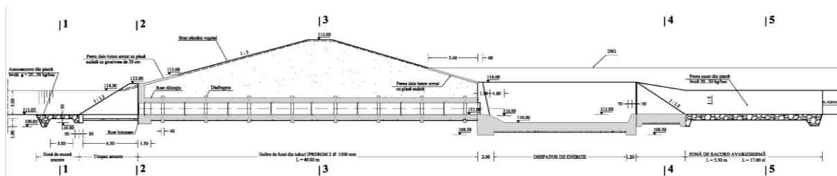
Fig. 4. Longitudinal section of the bottom outlet
