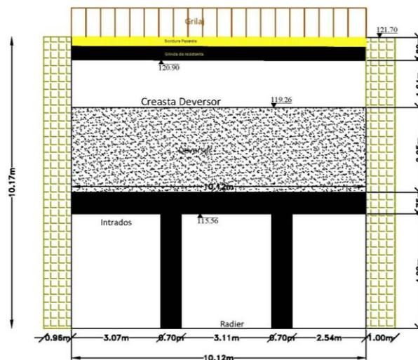
Fig. 2. Cross section of the transverse dam
