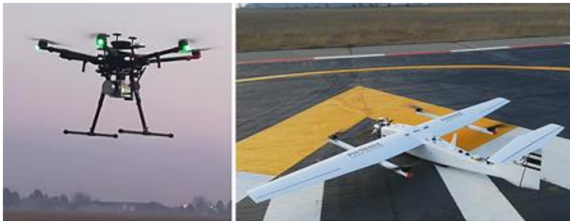
Fig. 1. LiDAR systems on DJI M600 PRO and Terrahawk CW-20
