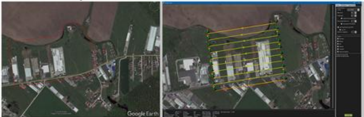
Fig. 5. Definition of the working area and planning of the mission
