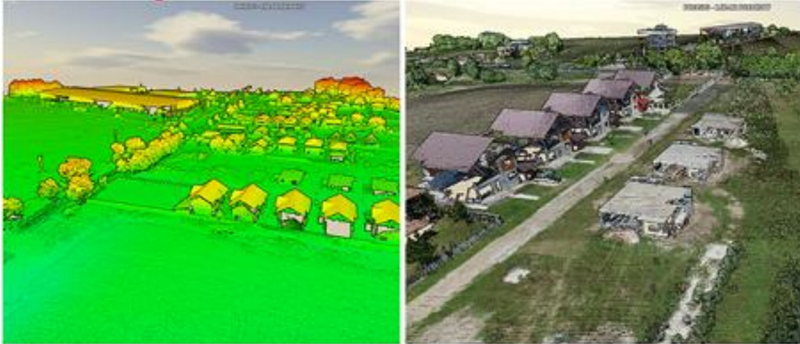
Fig. 10. Virtual 3D modelling without or with RGB information
