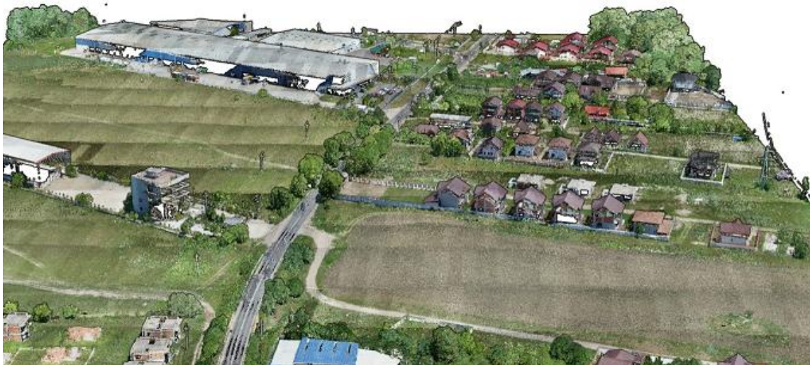
Fig. 11. Virtual 3D modelling using HQ Splats interpolation (Potree-Prosig)
