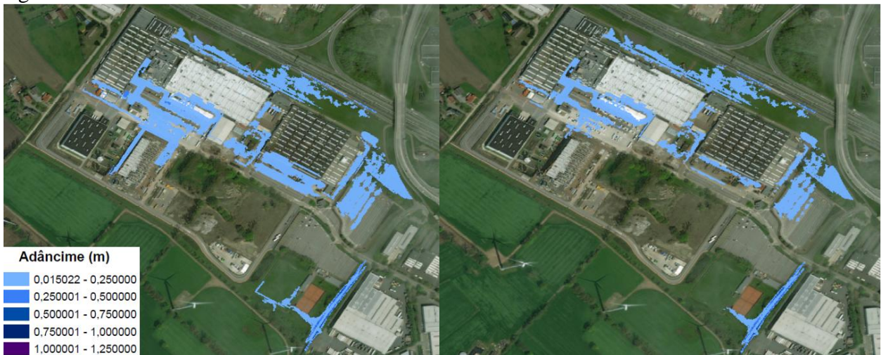
Fig. 8. Peak flood depth for one-in-two year’s probability: a) current situation b) proposed situation
