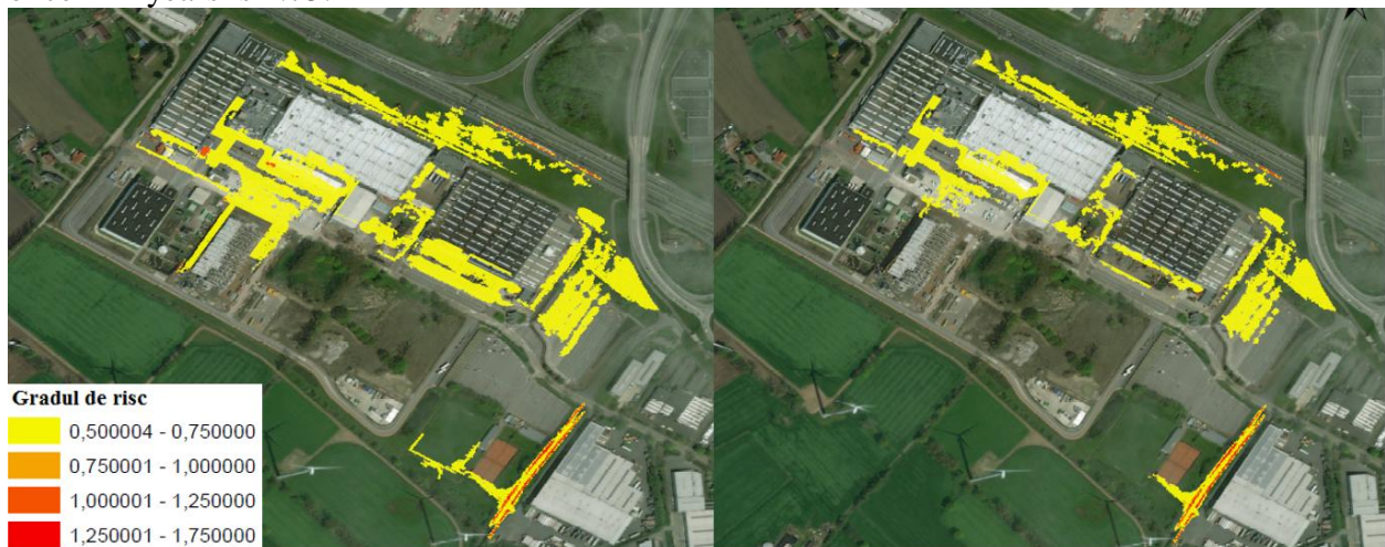
Fig. 10. Flood risk map for the one-in-two year's probability: a) current situation b) proposed situation
