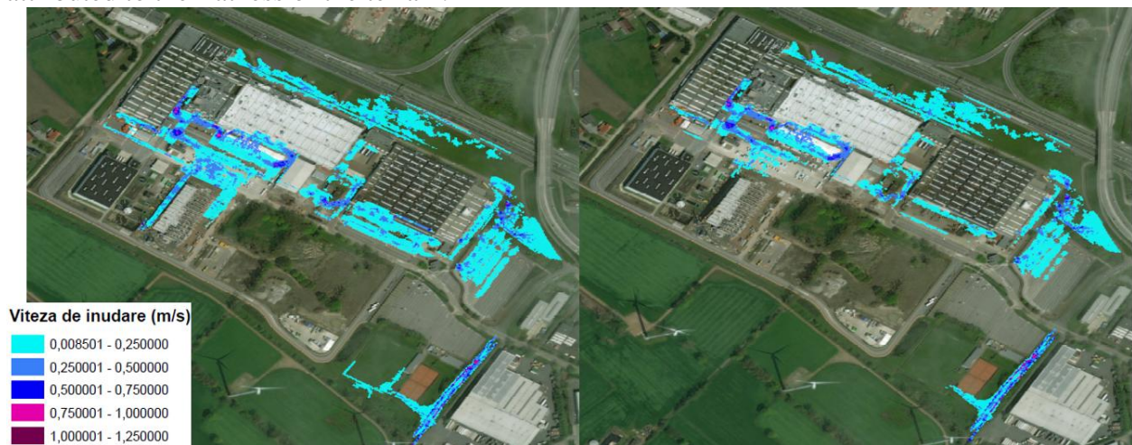
Fig. 9. Flood flow velocity for one-in-two year's probability: a) current situation b) proposed situation
