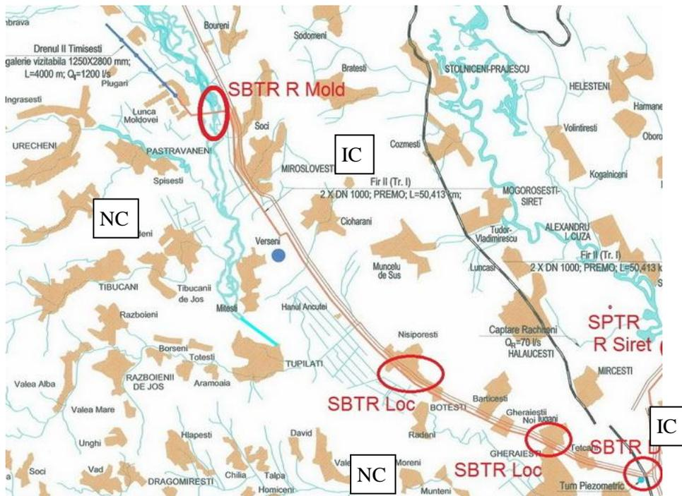
Fig. 5. Analysis plan of the Timișești - Săbăoani route of AdI + AdIIa + AdIIb + AdIII adductions from a real estate and urban water point of view: SBTR - undercrossing; NC - Neamț county; IC - Iași county
