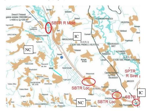
Fig. 5. Analysis plan of the Timişeşti - Săbăoani route of AdI + AdIIa + AdIIb + AdIII adductions from a real estate and urban water point of view: SBTR - undercrossing; NC - Neamţ county; IC -Iaşi county
