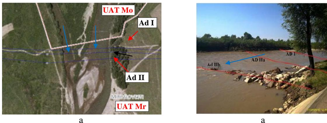
Fig. 6. The undercrossing area of the Moldova River by the Timișești - Iași Adduction: a - the orthophotoplan of the river undercrossing; b - view of the undercrossing area by the three pipes (Luca, 2012).
