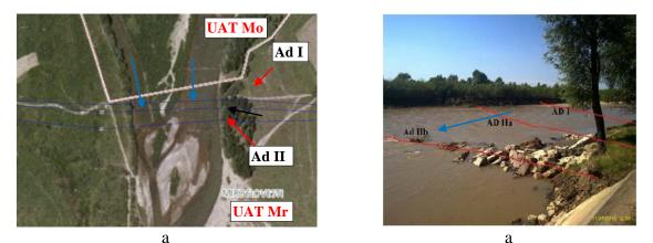
Fig. 6. The undercrossing area of the Moldova River by the Timişeşti - Iaşi Adduction: a - the orthophotoplan of the river undercrossing; b - view of the undercrossing area by the three pipes (Luca, 2012).
