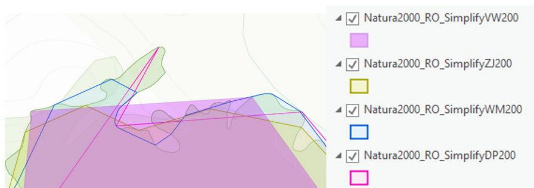
Figure 6 – Simplification applied on Protected Areas layer, v. 2019 - Bucegi Area (algorithms (Douglas-Peucker (DP), Wang-Müller(WM), Zhou-Jones (ZJ), Visvalingam-Whyatt(VW) – 200m)
