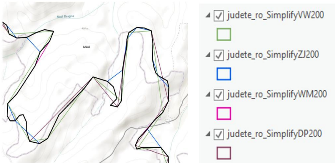
Figure 7 – Simplification applied on Counties layer - Salaj Area (algorithms (Douglas-Peucker (DP), Wang-Müller(WM), Zhou-Jones (ZJ), Visvalingam-Whyatt(VW))
