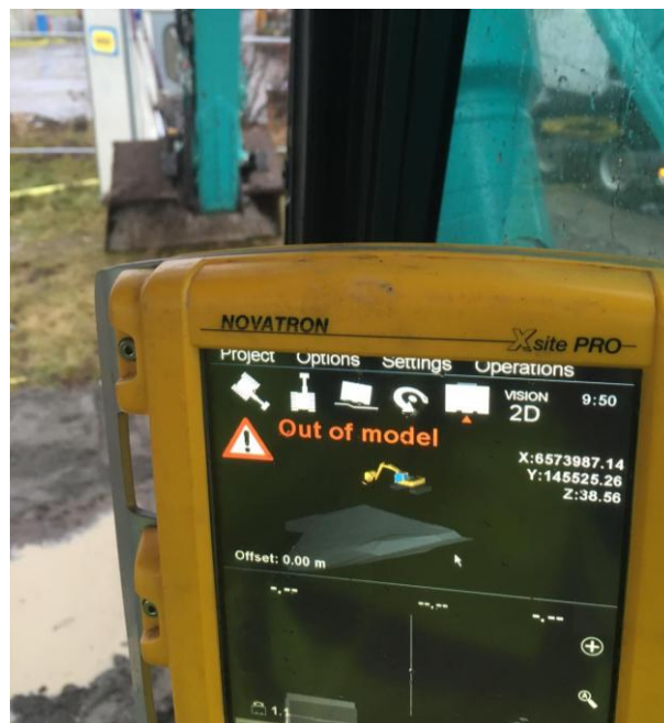
Fig. 7. Digital model used in production
