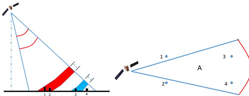
Fig.2. The spatial and azimuth resolution of SAR images
