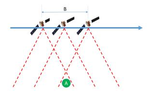
Fig.1. The principle of obtaining a synthetic SAR aperture
