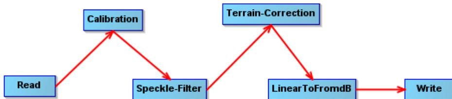
Fig.4.The steps of pre-processing process
