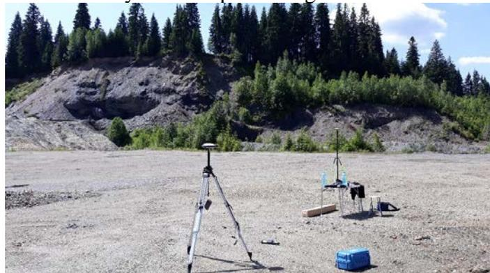
Fig. 2. Mounting the GPS station
