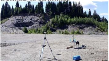
Fig. 2. Mounting the GPS station
