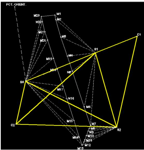
Fig. 3 Monitoring geodetic network
