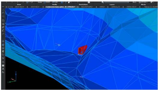
Fig. 8. 3D representation of the coastal gallery portal - horizon + 355m
