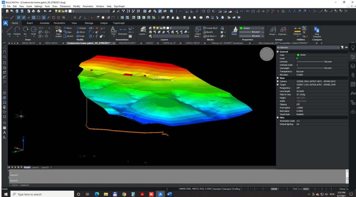
Fig. 7. 3D representation of surface land by MDT and underground mining works (aeration shaft and horizon gallery + 155m)
