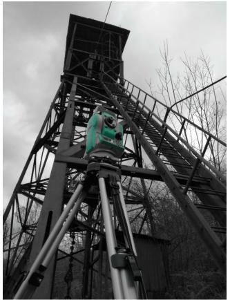
Fig. 2. Presentation of NIKON NPL 332 in the station, next to the aeration shaft equipped with extraction dispositive
