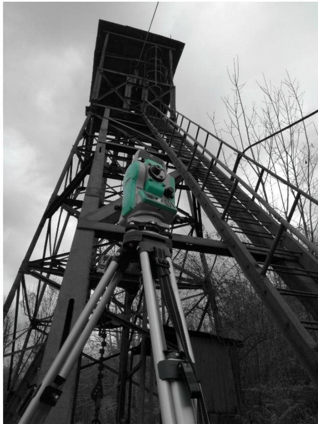
Fig. 2. Presentation of NIKON NPL 332 in the station, next to the aeration shaft equipped with extraction dispositive
