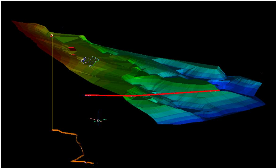
Fig. 9. 3D representation of surface land by MDT and underground mining works (aeration well, horizontal gallery + 355m and horizontal gallery + 155m)
