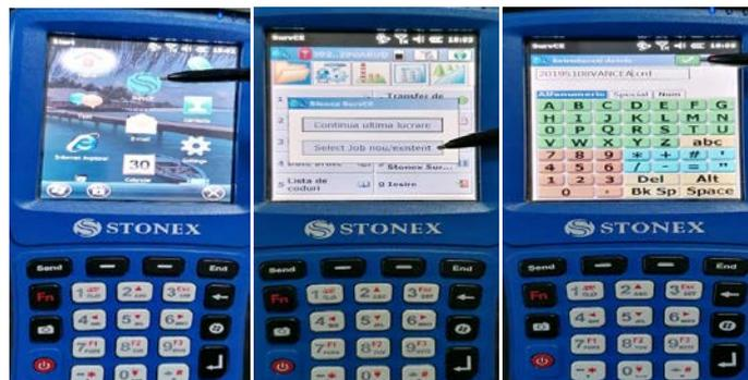
Figure 4. Setup and save of Job<sup>5</sup>
