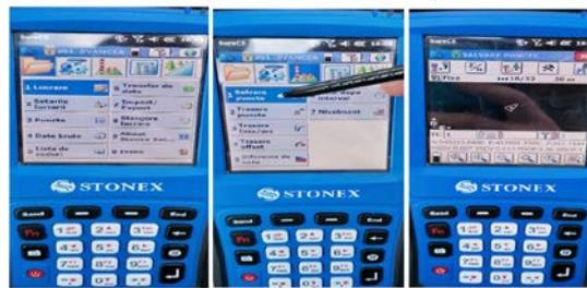
Figure 5. Registration of the first point<sup>6</sup>
