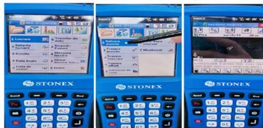
Figure 5. Registration of the first point<sup>6</sup>
