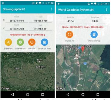
Fig. 7 Calculating the topographic orientation between two points and locating a point on the map [3]
