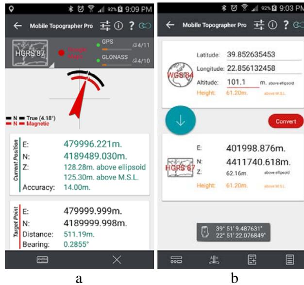
Fig. 4 Setting-out detail points in the field - a and converting points from one projection system to another - b [2]
