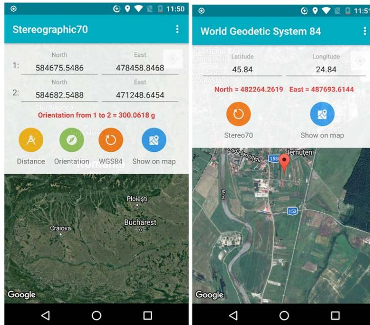
Fig. 7 Calculating the topographic orientation between two points and locating a point on the map [3]
