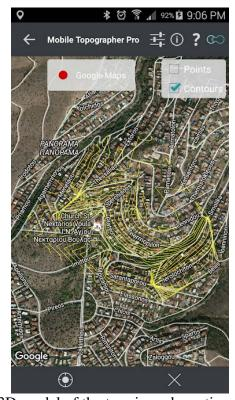
Fig. 5 Calculation of the 3D model of the terrain and creation of level curves [2]
