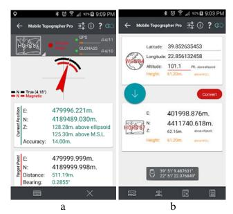
Fig. 4 Setting-out detail points in the field - a and converting points from one projection system to another - b [2]
