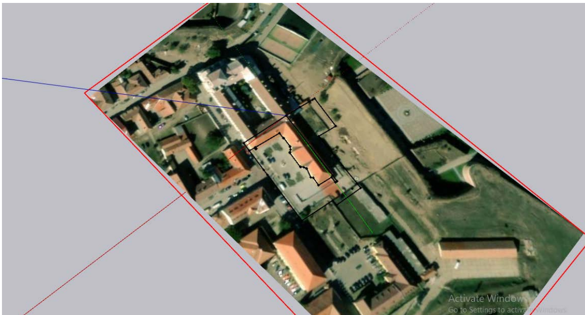
Fig. 4 Modeling in Google SketchUp, based on the digital terrain model imported from Google Earth and topographic plan imported from AutoCAD
