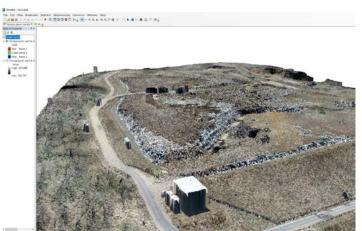
Fig. 8 Three-dimensional visualization of the orthophotoplan in ArcScene software
