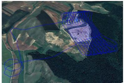
Fig. 3. Software-Arial Imaging- Planned trajectory for UAV UX5HP
