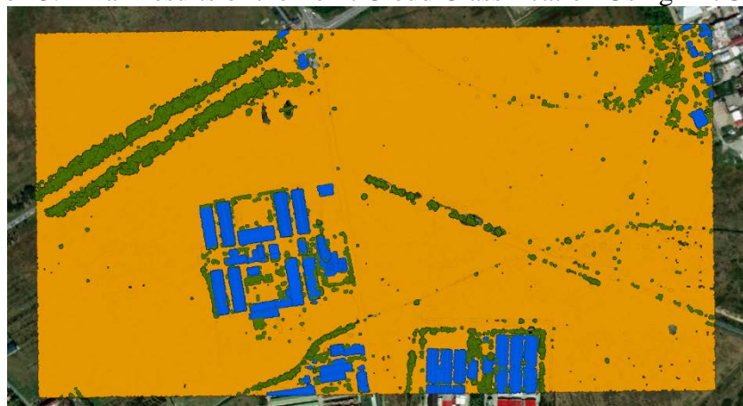
Figure 24. Final Results of the Point Cloud Classification Using ArcGIS Pro (Ground-Orange, Buildings-Blue and High Vegetation-Green)
