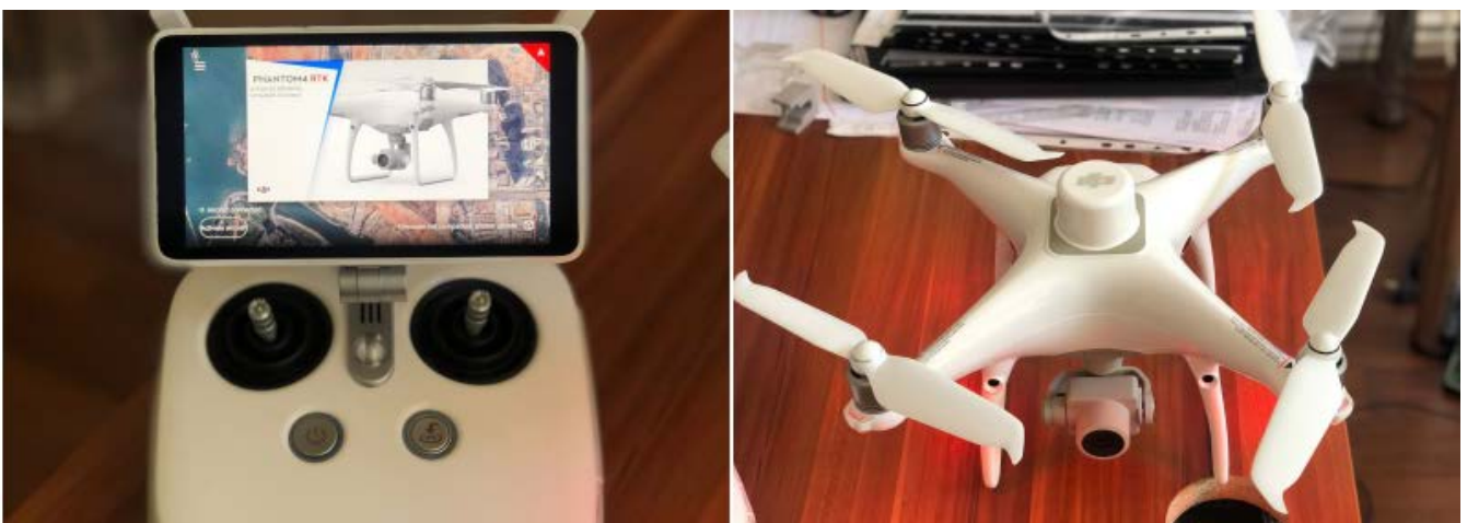
Fig. 2 – The drone used for flight (DJI Phantom 4 RTK)
