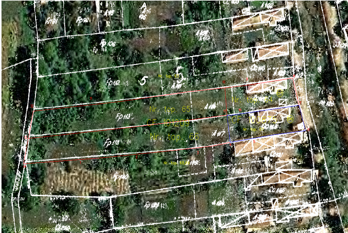
Fig. 5 Extract from Curciu cadastral plan, overlap with the cadastral plan resulting from measurements and with the related orthophoto plan of the area
