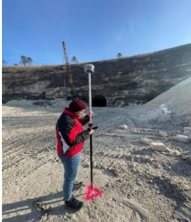
Fig. 2. Measurements with CHCNAV I50 GNSS receiver
