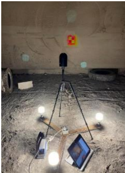
Fig. 4. One of the optimal stations of the Leica BLK 360 scanner.
