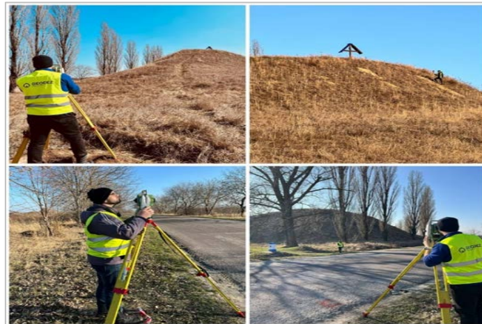
Fig.4. Land work -total station data acquisition
