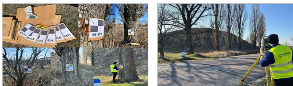
Fig.5. Fixing and measuring the orientation markers
