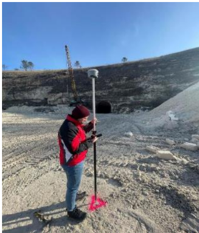
Fig. 2. Measurements with CHCNAV I50 GNSS receiver
