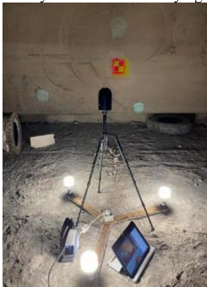
Fig. 4. One of the optimal stations of the Leica BLK 360 scanner.
