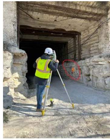
Fig. 3. Measurements with Leica Viva TS15 total station
